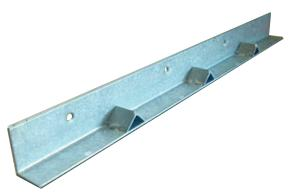
The maximum slope of the roof construction without stops shall be 7:12. Roof construction with slopes greater than 7:12 but not more than 12:12 shall have stops of a minimum 3 inch  $\times$  3 inch  $\times$  1/4 inch (76 mm × 76 mm × 6 mm) steel plate welded to the angle at 24 inches (610 mm) on center along the angle or as approved by the building official.
